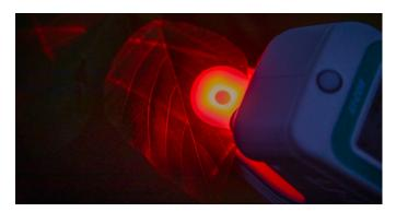
For dark-adapted leaves, the LI-600 measures maximum quantum yield  $(F_{\nu}/F_m)$ , or the maximum proportion of absorbed light that can be used to drive electron transport.  $F_{\nu}$  is variable fluorescence yield in a dark-adapted leaf;  $F_m$  is maximum fluorescence yield in a dark-adapted leaf;  $F_o$  is minimum fluorescence yield in a dark-adapted leaf.
