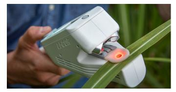
For light-adapted leaves, the LI-600 measures the quantum yield of fluorescence ( $\Phi PS_{II}$ ), which is the proportion of absorbed light by photosystem II that is used for electron transport.  $F_m$  is maximum fluorescence yield in a light-adapted leaf;  $F_s$  is steady-state fluorescence yield in a light-adapted leaf.
