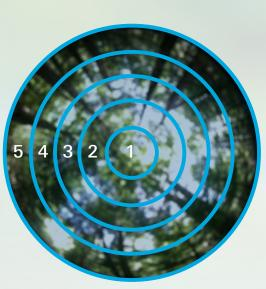
The approximate field-of-view of each ring is simulated by the fisheye photo (above), where concentric circles represent the five view angles.
