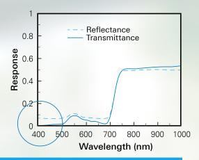
The 490 nm filter minimizes the contribution of radiation scattered by the foliage, which is very low below 490 nm. The detector in the optical sensor responds from approximately 320-490 nm (circled region).
