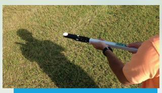
Using an optical sensor with diffuser cap to measure sky radiation properties for light scattering correction.
