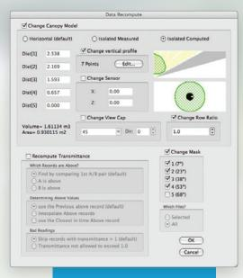
The FV2200 recompute interface, showing a masked outer view ring.
