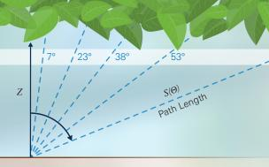
The path length of the optical sensor's view through a full cover canopy varies by view angle.
