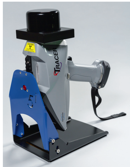
TRACER 5 desktop stand kit with safety shield in place
