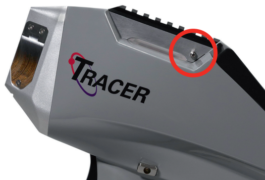
Port connection (red circle) to purge with helium
