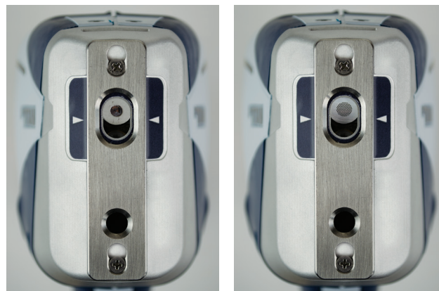
S1 TITAN with punctured detector (left) and undamaged detector (right) when fitted with the TITAN Detector Shield™.
