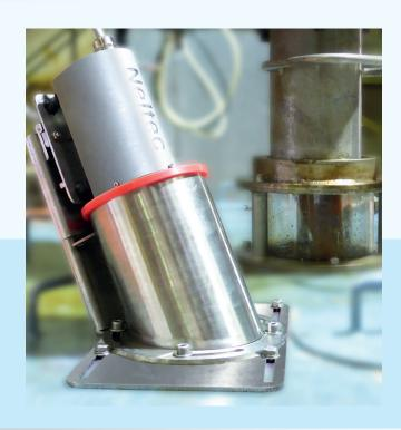
The ColourQ 1700 CC is a colour indicator for installation on continuous centrifugals in order to indicate the colour of the crystals just before they leave the screen. If the colour is too high, too much colour is sent back in the process, while a low colour means too much sugar is being dissolved.
