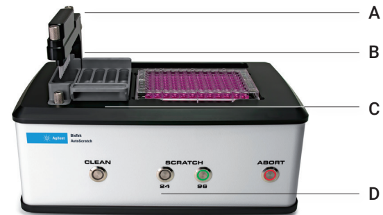
Figure 5. The Agilent BioTek AutoScratch wound making tool features: (A) 8- or 4- pin manifold with replaceable tips (B) Manifold arm, designed for easy manifold exchange (C) 4-trough cleaning and decontamination station (D) Simple control panel
