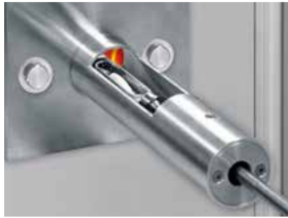
Manual introduction of the sample into the furnace through the loading head
