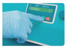
**Step three**Load the rotor and start centrifugation
