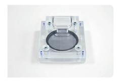
**Step one**Mount the ZentriForm insert: Insert the master and O-ring and screw the mould together
