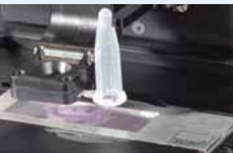
A Prepare sample directly on mmi Membrane Slides
