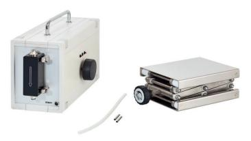
The aerosol flow is split by a precision capillary into a sample and bypass flow. In the bypass flow, all particles are removed by the built-in highefficiency HEPA filter capsule. Downstream, both flows are mixed again. The actual dilution ratio is monitored by measuring the differential pressure over the capillary.
