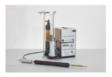
The variable two-stage diluter operates with recirculated conditioned air. All process air is generated by the ESS. No compressed air supply is required.
