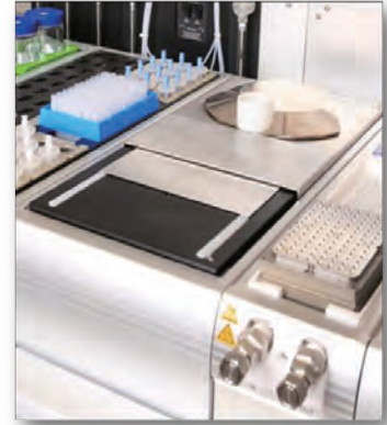
3. Balance with Integrated Camera 天平和摄像头
