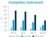
CVs measured with various flow rates
