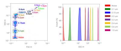
NIST particle size standards run on NovoCyte Advanteon displayed in a two-dimensional density plot or as a histogram showing the SSC resolution down to 0.1 um.
