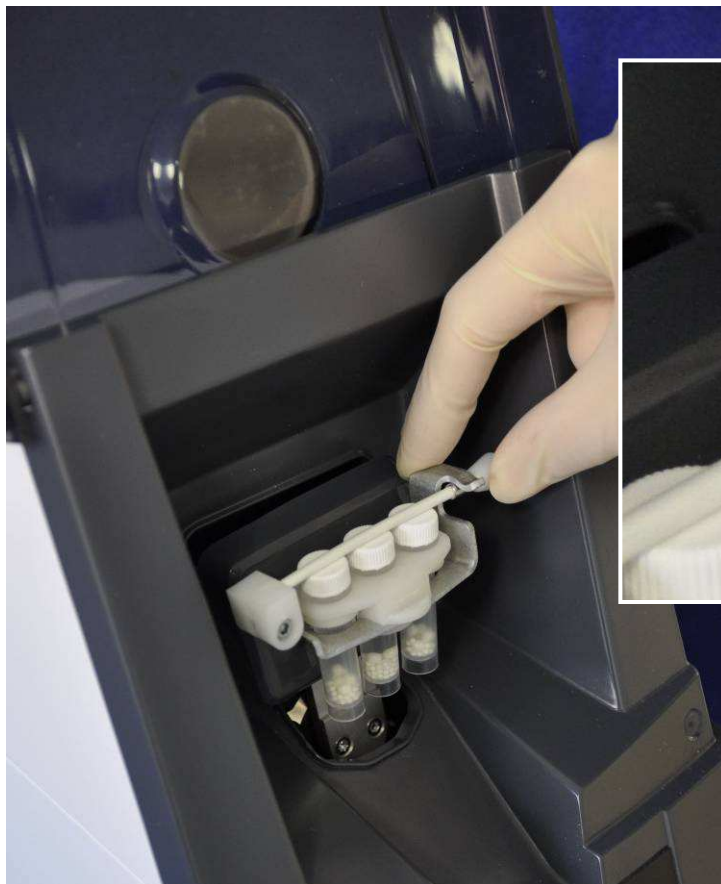
Tube blocking rod locked position
