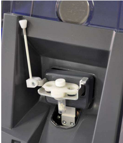
Correct and only position for 1 tube
