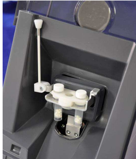
Correct and only position for 2 tubes
