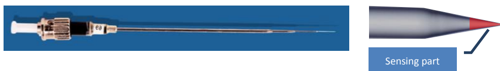
Figure 2 - A probe (left) and its sensing part (right)
