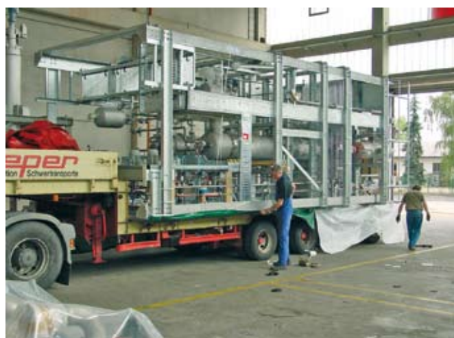
Loading of a skid-mounted plant with 2 Short Path Distillators (4 m 2 evaporation surface area each)
