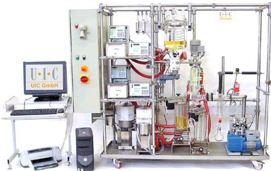
KDL 5 CADi for automated routine distillations
