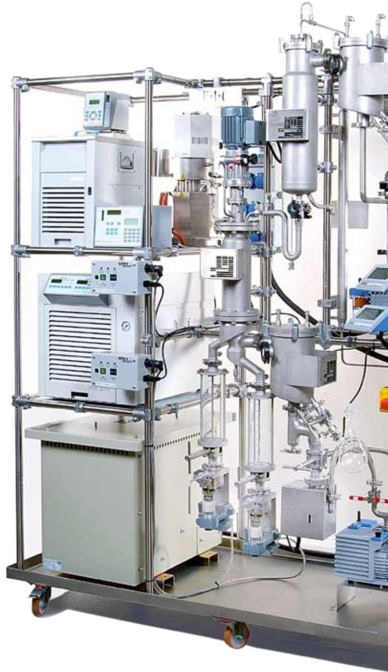
KD 6 pilot plant with degasser and Short Path Distillator
