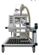
Liquids, solids and melts can be filled into vessels with the formulation and filling system featuring freely programmable mixing ratios.
