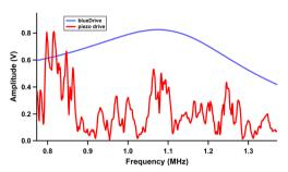
Tune of a small, fast Nanoworld USC-F1.5-k0.6 cantilever driven with blueDrive in water closely matches the theoretical response, while the piezo-driven response has multiple peaks.
