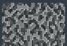
**4-level beam splitter**Cell width/depth 500nm
