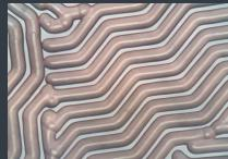
**Micro-engraving** Line width 2Oμm, depth 1Oμm Courtesy of Karmic Sàrl
