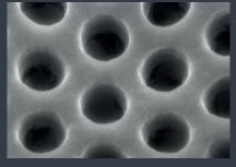
Nanostructure for life science Cavity diameter 35Onm Courtesy of IMT AG
