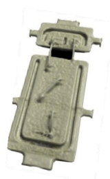
1.5 mm LED reconstructed using KA Imaging's inCiTe™ micro-CT.
