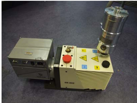
Figure 113 - Varian external filter fitted to Varian rotary pump
