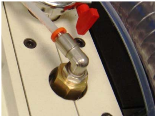
Figure 111 - Installed oil return fitting on the Varian rotary pump
