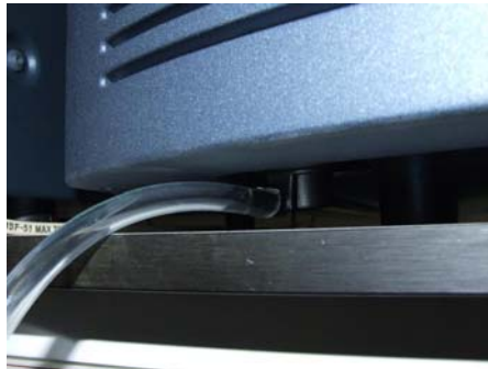
Figure 5 - Liquid waste line connection
