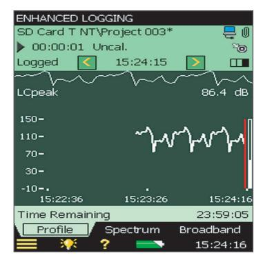
With Sound Recording software, you can initiate a sound recording manually, automatically using level triggers (both broadband and frequency based level triggers) or at set time intervals. Pre-recording lets you record sound occurring before sound recording is triggered, and memory space is saved by setting a suitable recording quality and maximum duration.
