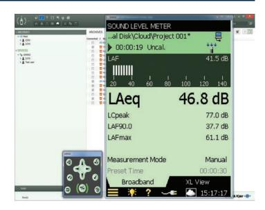
When the logger is used with Noise Monitoring software, it can be used with Noise Sentinel™ and Noise Sentinel On Demand. Noise Sentinel is a Web-based subscription service that provides continuous, real-time monitoring and compliance management. It provides audio playback for investigation and comprehensive reporting provide a traceable record of regulatory compliance.
