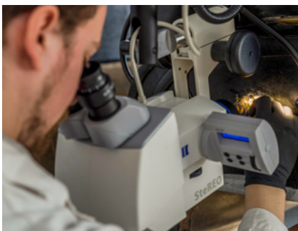
Images 5 & 6 The ZEISS SteREO Discovery.V8 stereo microscope with a floor stand enables conservators to work sitting down comfortably even with larger objects.
