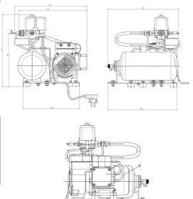
Control and safety devices with pressure switch, non-return valve, pressure gauge, safety valve and mechanical condensate drain outlet\*
