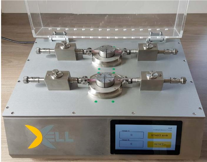
Twin folding tester with new Touch screen display
