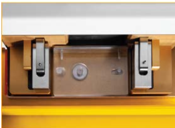
Water bath between the clamps
