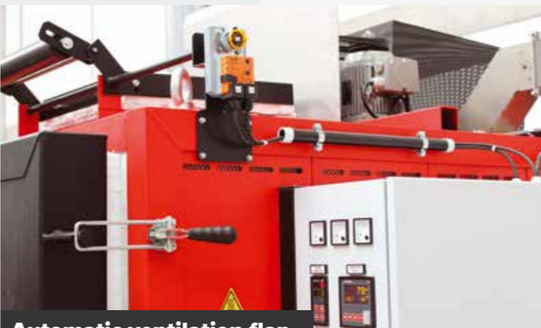
Automatic ventilation flap
