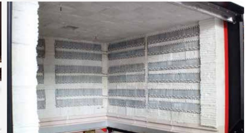
Resistance heating – meandres
