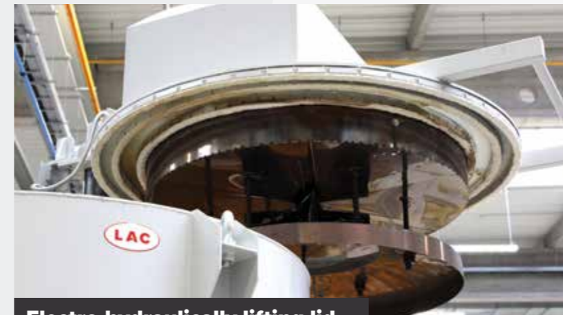
Electro-hydraulically lifting lid
