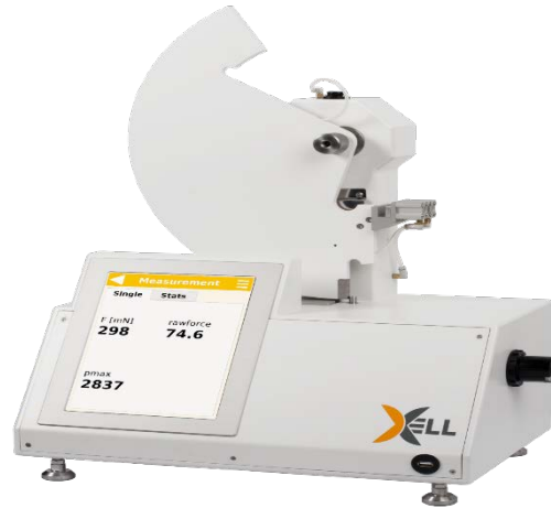
Elmendorf tester with 8.000 mN pendulum
