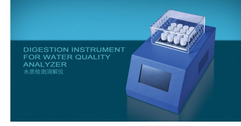
XJ-16型消解仪可用于COD、总氮、总磷等水样的消解预处理,具有加热速度快,加热均匀,恒温,定时等功能。 XJ-16 Digestion Instrument is used for the digestion of water samples in the pretreatment before water quality analysis (eg. testing COD, total nitrogen, total phosphorus etc). The instrument has fast heating function and can heat samples evenly. It also has thermostat and timing functions.
