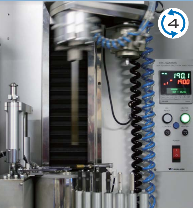
The Chuck on the Robot Arm Grabs up the Piston and Inserts it into the Cylinder
