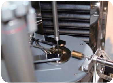
Cleaning the Die with 2 Different Die Cleaning Rods
