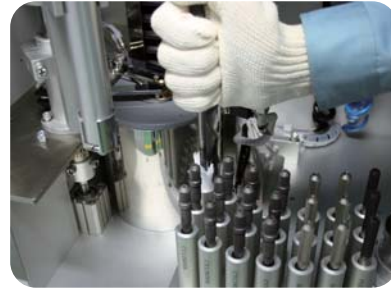
Set the Cylinder Cleaning Rod with the Gauze Attached to the Rod Holder
