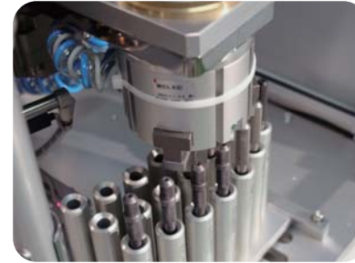
The Robot Arm AUTOMATICALLY Choses the Cleaning Rod to Clean the Cylinder
