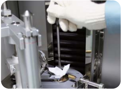
Attach the Gauze to the Cylinder Cleaning Rod using the Heat of the Cylinder
