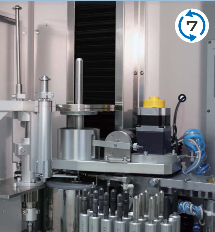
The MVR or the MFR Value is Automatically Measured and the Data is Transferred to the PC Software
