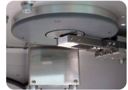
The Die Tip Top Cleaning Scissor to Wipe off the Sample on the Tip Top of the Die Cleaning Rod
