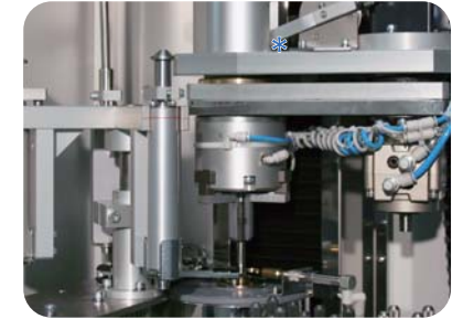
The Robot Arm Repeatedly Twists and Elevates to Clean the Cylinder (Maximum 4 times)
