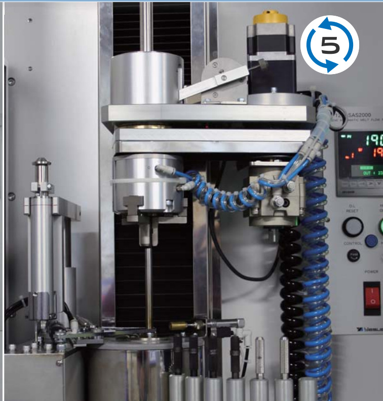
The Up and Down Movement of the Robot Arm Pushes in the Sample to the Starting Position
