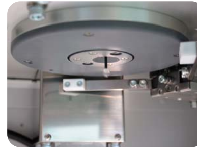
The Die Tip Top Cleaning Scissor to Wipe off the Sample on the Tip Top of the Die Cleaning Rod
