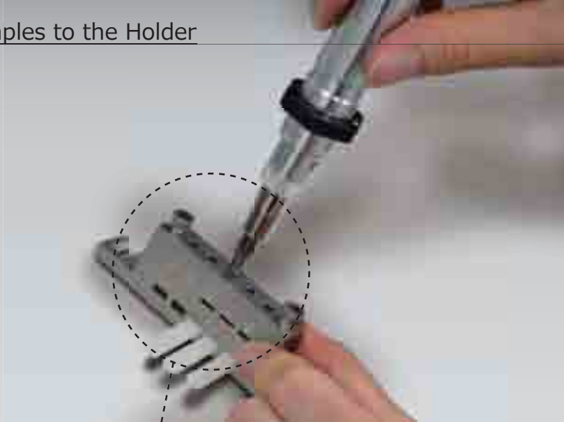
Attaching the Test Samples to the Holder using the Torque Wrench
