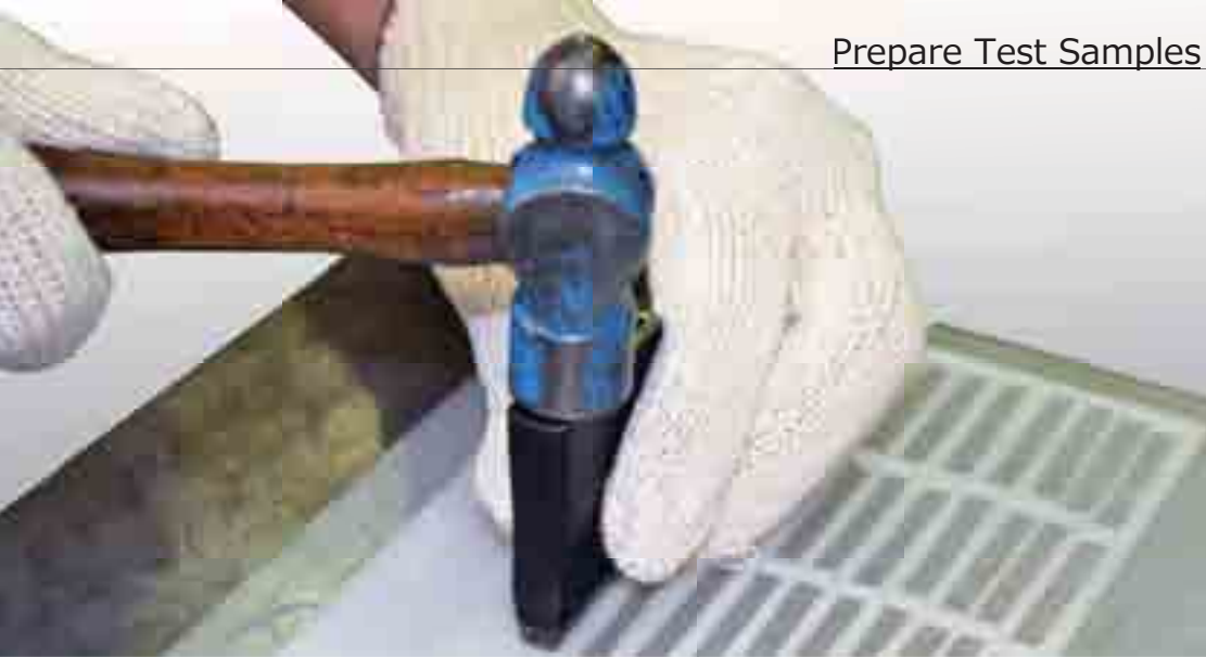
Knocking the Sample Sheet with a Hammer and Specimen Cutter
