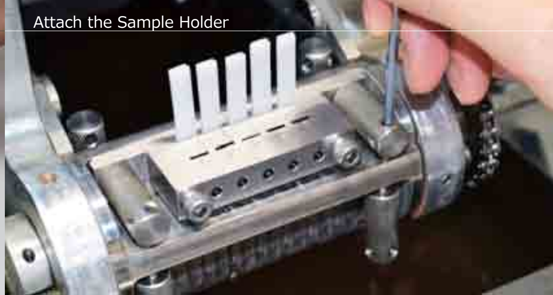
Attaching the Holders to the Rotary. Maximum 4 Holders can be attached to the Rotary.
