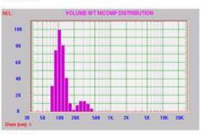
In this case, the peaks shifted to even smaller sizes when the gel temperature was raised to  $40^{\circ}$ C for 15 minutes. The second peak's center of mass began shifting to smaller sizes as well.
