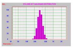
Starting conditions: The gel is filled with water at room temperaure (26°C). When the temperature is raised to 40°C, the polymer gel will collapse upon itself, and the size will drop to approximately 100nm.
