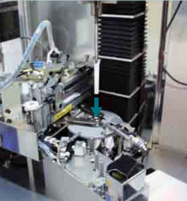
The Cylinder Cleaned Automatically with the Cylinder Cleaning Rod >>>
