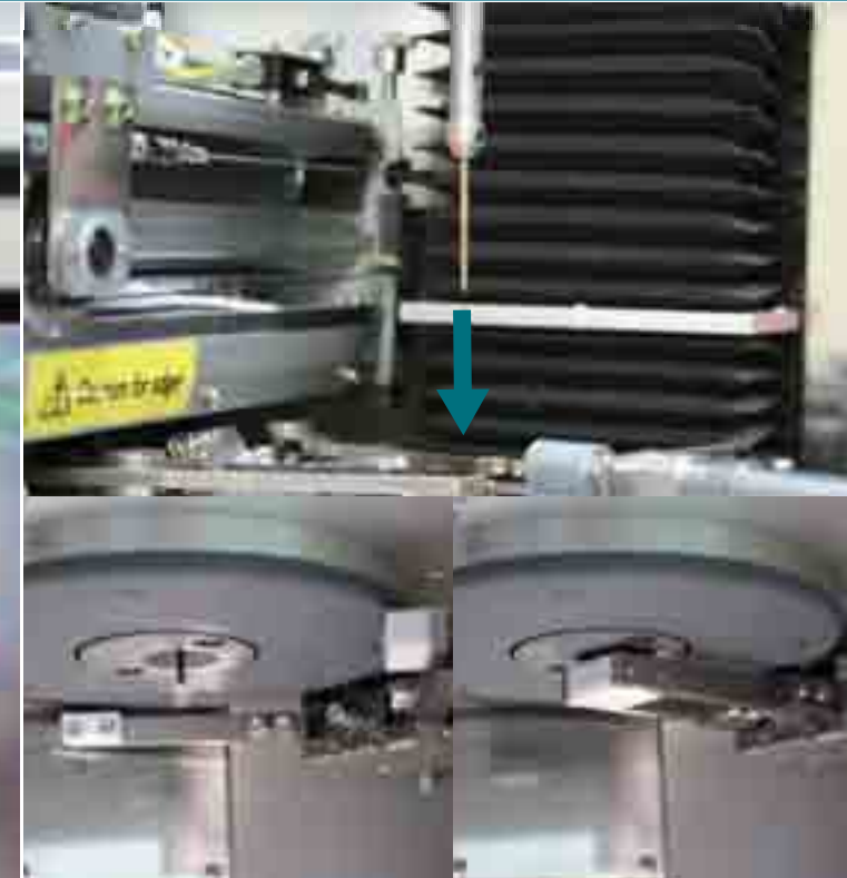
The Left over Sample in the Die to be Cleaned Automatically with 2 Different Die Cleaning Rods
