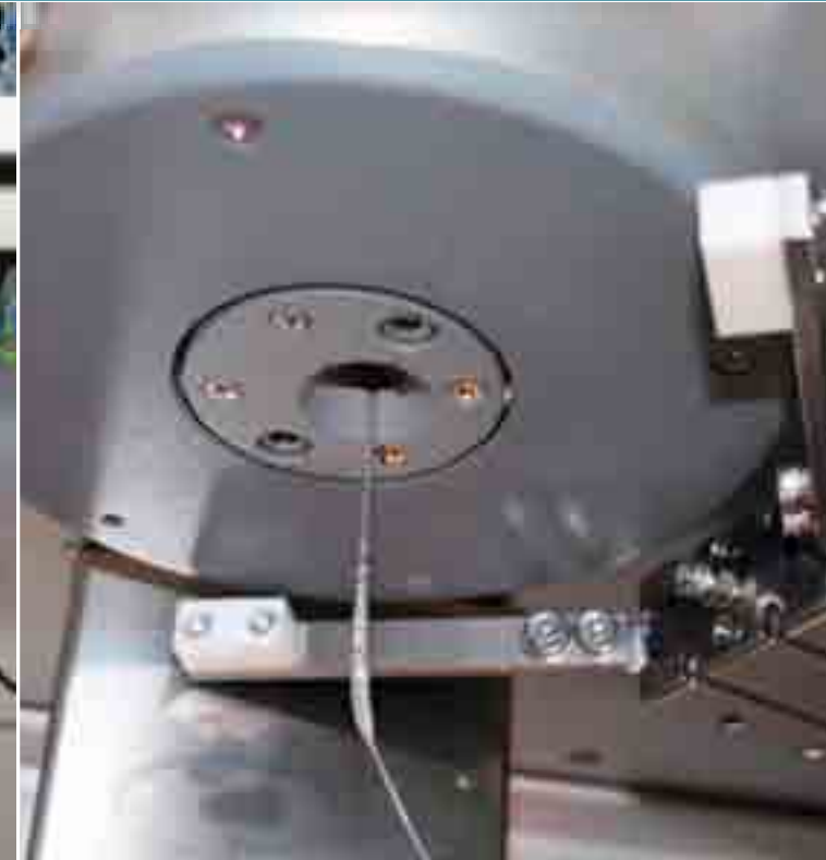
The Pushed out Sample Flows out from the Die
