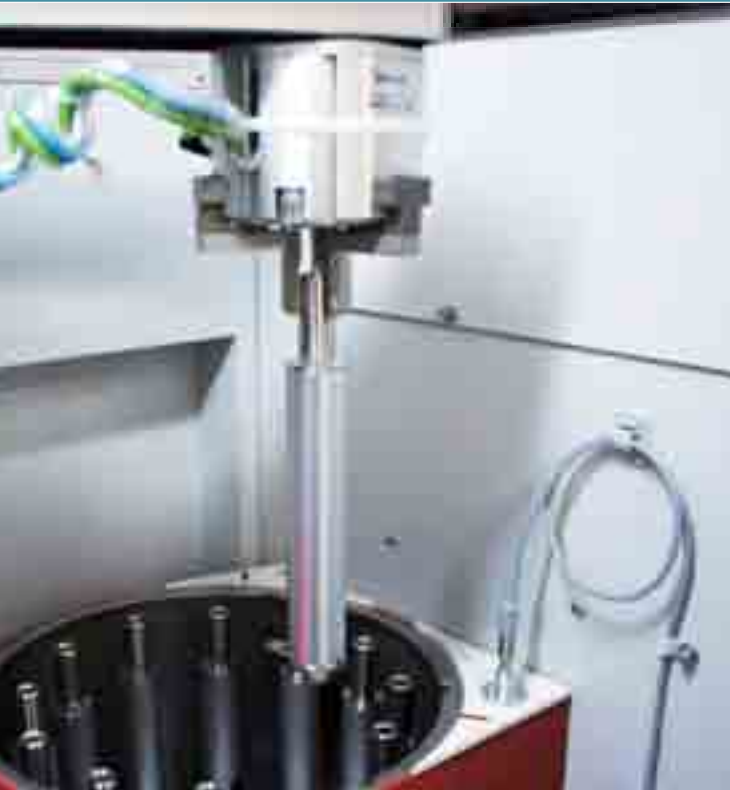
The Robot Arm will Automatically Pick Up the Sample Cup
