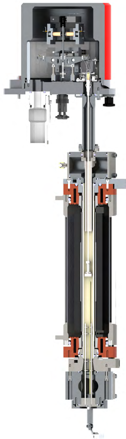
SCHEMATICS OF THE THEMYS BALANCE, FURNACE AND TEMPERATURE CONTROL
