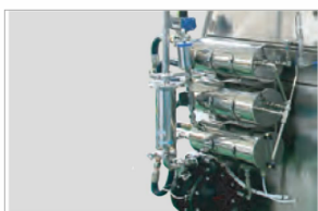
Solution tank to prevent the solidification 原料放凝固装置
