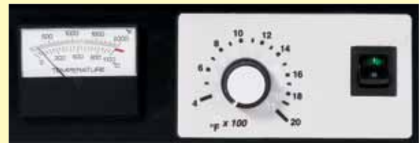
Analog prometer displays temperatures on LMF-A550 models.
