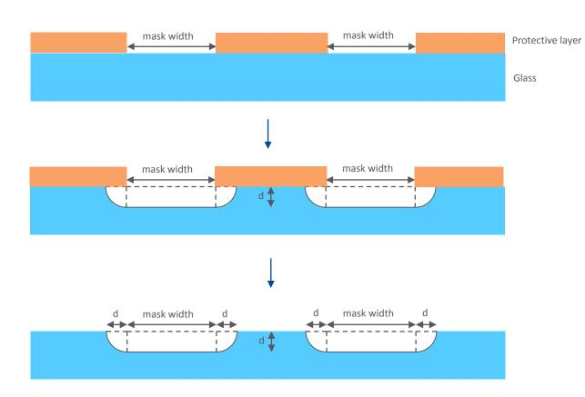
Due to our processing method, the channels always have the shape depited here. We expose a piece of glass to acids that desolve the glass equally fast in all directions. Because of this 'growing in all directions', the corners of the channels are round and the bottom width of the channel is smaller than the top width.
