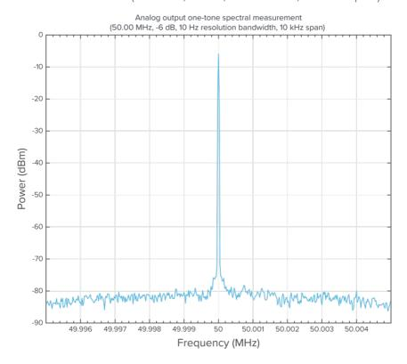
One-tone spectral measurement (50 MHz, -6 dB, 10 Hz RBW, 10 kHz span)
