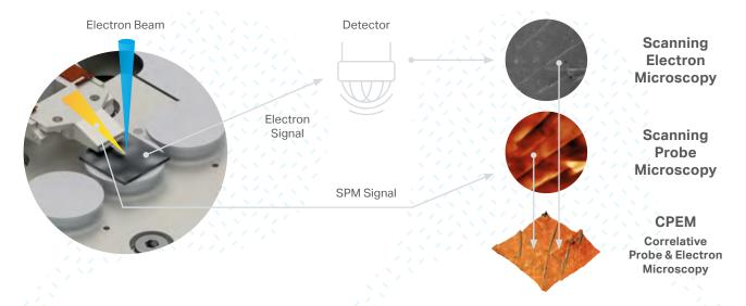
CPEM technology enables correlative imaging of the standard SEM and SPM methods in a manner that has not been available until now.
