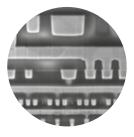
SEM image Logic Device – 65 nm technology. Source: FEI Company
