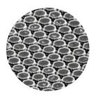
SEM image Hexagonal pattern etched in silicon during optical exposure of the photoresist. Source: FEI Company
