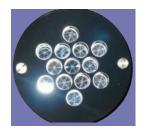
The Model 4500 MkIII uses a highly homogenous advanced **LED light source** and a glass multi-prism **retro-reflector** to reduce the effects of misalignment on the measured opacity, thereby achieving the lowest possible detection limit. The **Flood LED** technique eliminates the requirement for continuous moving parts (chopper motors etc). Collectively these features provide the highest level of stability and lowest level of optical and electronic drift available.
