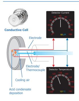
An acid film, such as sulphuric acid, is a good conductor of electricity. If a surface bearing two electrodes is introduced into a gas containing sulphuric acid vapour, any condensate forming on the surface would soon be detected by a current flowing between the electrodes.
