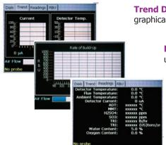
Trend Display - Shows detector current and temperature on a rolling graphical display.
