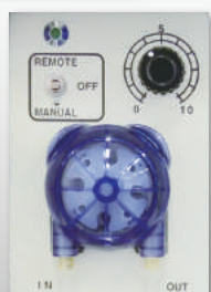
Chemical suppressor pump unit
