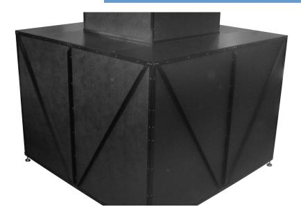
Sciencetech's flash solar simulators are designed to test large photovoltaic devices up to  $2m \times 2m$  (79"  $\times$  79") in size. It uses a heavy duty xenon flash lamp and AMI.5G calibrated solar filter to approximate the sun's true spectral distribution following ASTM E927-05 (2005) Class A standards. The simulator fires short flashes of light to avoid heating a photovoltaic device for measuring its performance.
