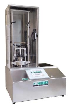
The Dome Reversal Tester is a semi-automated buckle tester designed to determine the exact pressure at which the bottom dome of a can begins to buckle.
