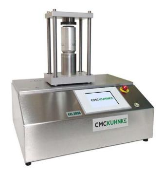
The easy-to-use AXL-3050 tester measures the axial load resistance of beverage cans.
