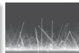
Si nanowires using Au NP as catalyst
