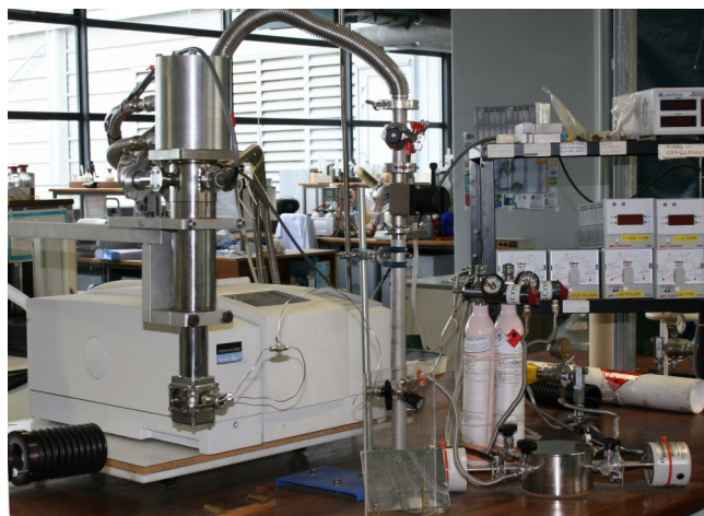
System set up for Matrix Isolation. Mixing chamber lower right. Expander and sample can be manually rotated with respect to the shroud and window. Clamped shroud stays stationary during sample rotation.
