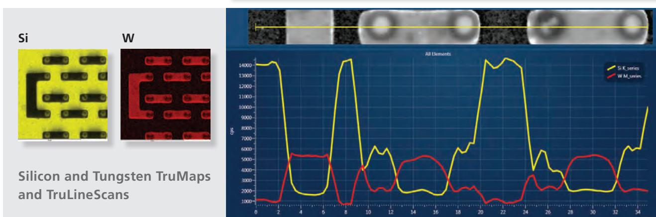
Standard X-ray Maps and LineScans indicate that Tungsten and Silicon are concentrated in similar regions of the structure, however, with TruMap technology the real positions of these elements are revealed.
