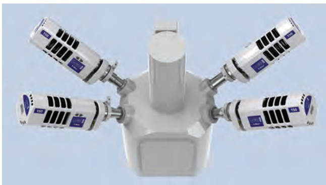
A configuration with four X-Max N 150 detectors - together making up a system with an overall effective area of 600 mm 2 .
