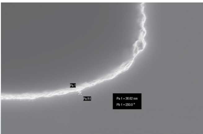
Highly conformal and uniform PEALD TiN + Cu films on high aspect ratio trenches.
